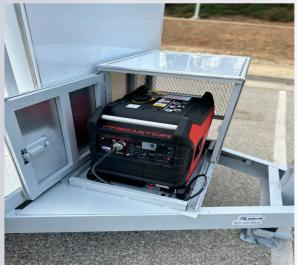
We installed axles of 71000 LB each for a load of 14000 LB with 235 radial tires. We manufacture and adapt a special box for the generator that protects and offers easy check of the generator.
