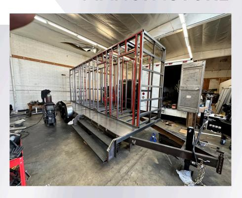
We star ted the manufacture of our rest room trailers with focus on metal structure of tubes and chanel, heavy and comfortable structure for good performance.
